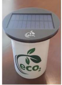
**B- Multiple mode**: using NB-IOT (narrow band IOT) technology to establish a network between the sensors and a centralized device. In this case, only the central device
